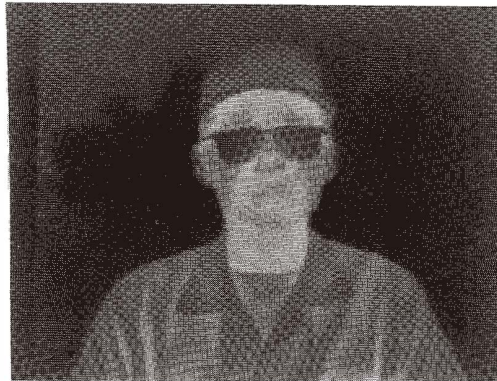
Fig. 9. Infrared image obtained from 320×240 YBaCuO microbolometer FPA.
