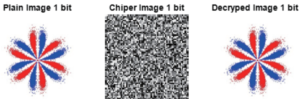
Fig. 8. (Color online) 1-bit encryption and decryption for wind turbine gearbox tooth-break fault vibration feature snowflake image.
