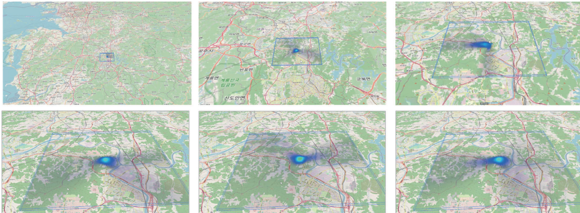
Fig. 11. (Color online) Atmospheric dispersion modeling results in the digital twin area of 13 \text{ km} \times 13 \text{ km} \times 200 \text{ m} for one year.
