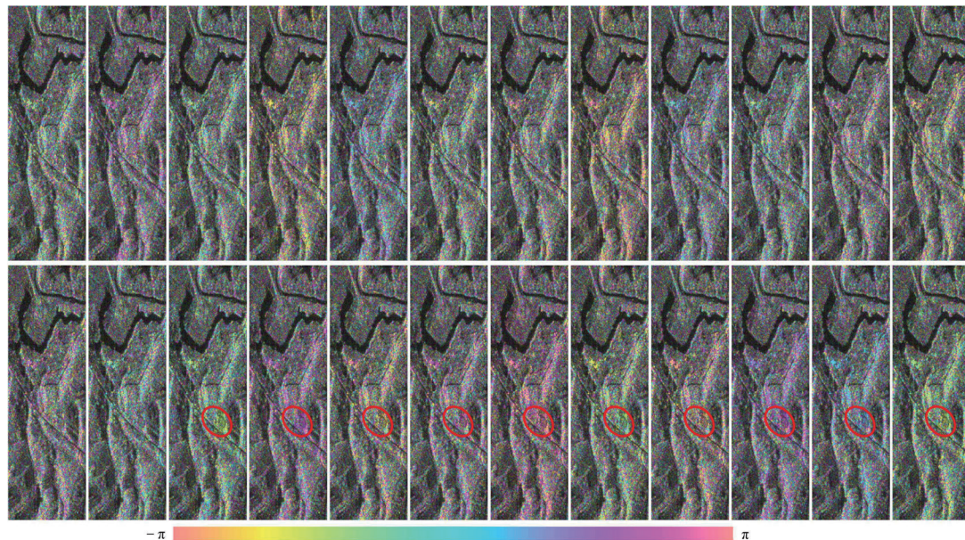
Fig. 7. (Color online) D-InSAR results acquired from ALOS-2 PARSAR2 images. The location of the highway slope is indicated by the red outline. We only drew the red outline in the interferogram after October 28, 2018.
