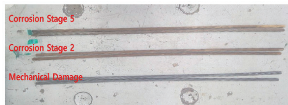
Fig. 1. (Color online) Corrosion and mechanical damage specimens.
