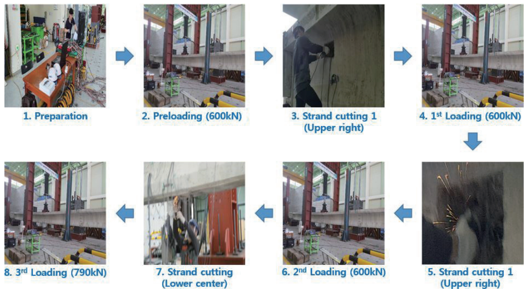
Fig. 8. (Color online) Test procedure for internal tendon destructive of I-type PSC structure.
