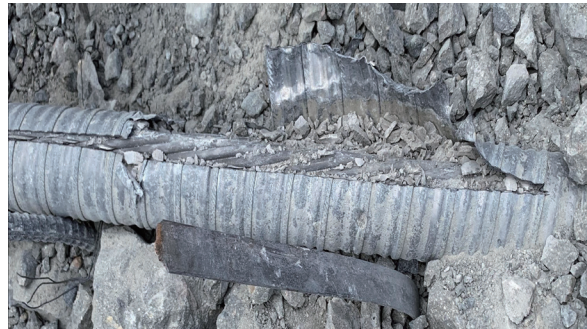
Fig. 16. (Color online) Specimen inner tendon after load test.
