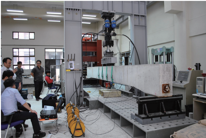
Fig. 3. (Color online) PSC structure defect detection experiment.
