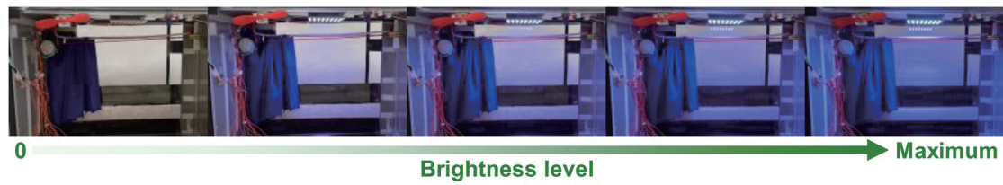
Fig. 6. (Color online) Brightness adjustment test of the RGB LED matrix.
