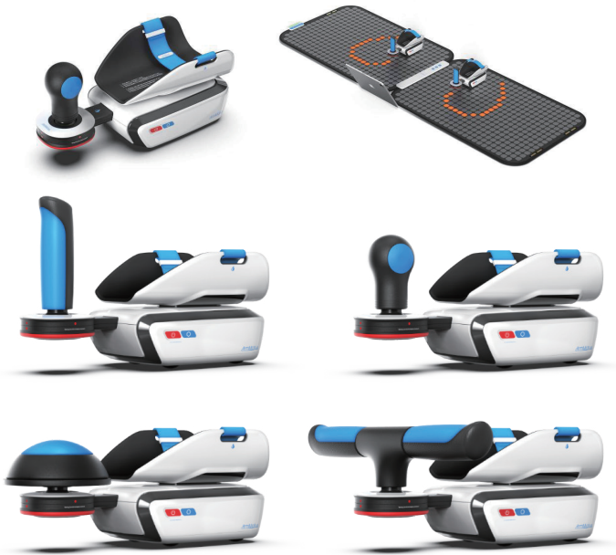
Fig. 11. (Color online) Rendering of home-based rehabilitation robot for patients with upper limb hemiplegia.
