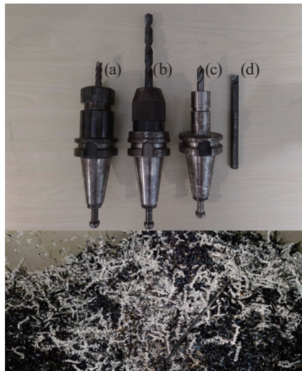
Fig. 1. (Color online) Machining tools used in this study: (a) four-flute end mill, (b) twist drill, (c) 45° chamfering tool, and (d) internal turning tool (from left to right).
