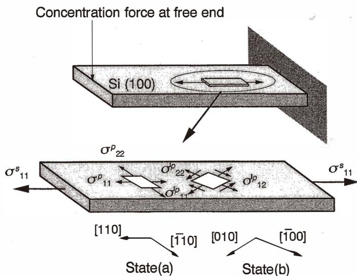
Fig. 4. Stress states of poly-Si piezoresistors on Si cantilever subjected to bending.
