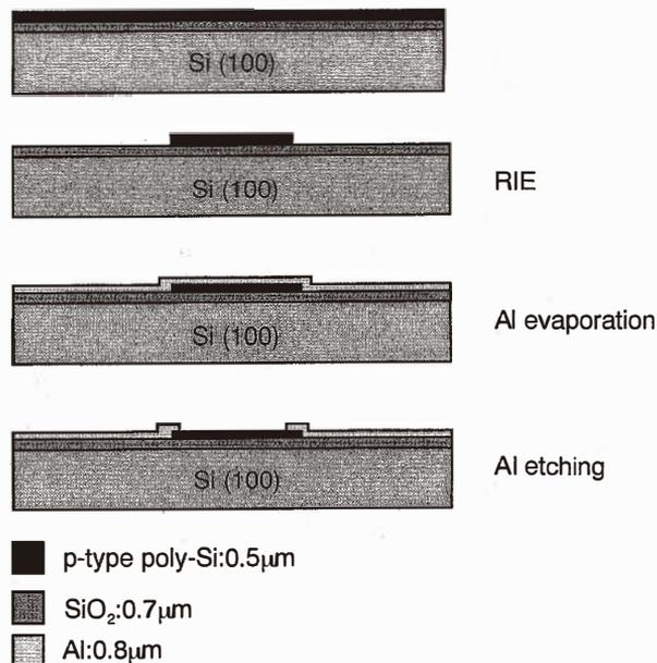
Fig. 1. Fabrication process of p-type poly-Si piezoresistor.
