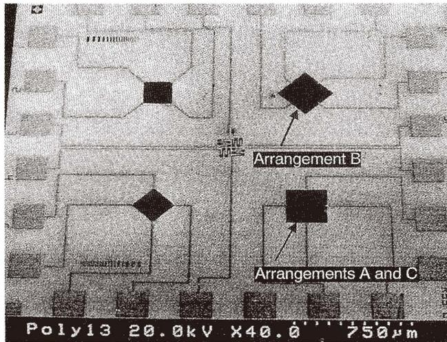
Fig. 3. Fabricated p-type poly-Si piezoresistors.
