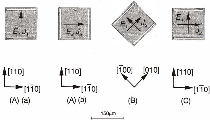
Fig. 2. Schematic top-view of fabricated piezoresistors.
