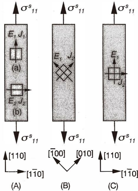
Fig. 5. Arrangements of poly-Si piezoresistors.
