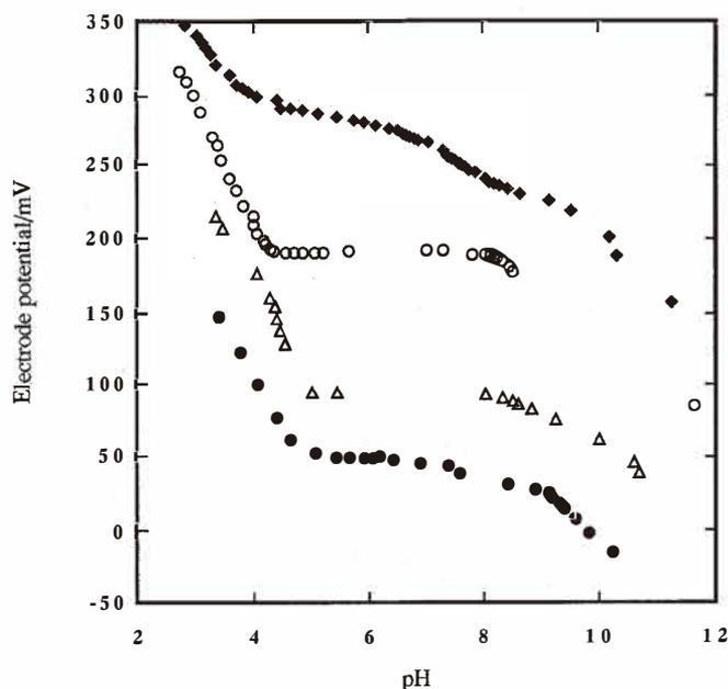
Fig. 8. Effect of pH on the potential of the electrodes. A sensing membrane was prepared using  $\text{Ag}_2\text{S}$ -coated  $\text{NiS}$  particles at a coating time of 2.5 h (electrode 2). Concentration of  $\text{Ni}^{2+}$ ,  $\blacklozenge$ :  $10^{-1}$  M;  $\circ$ :  $10^{-2}$  M;  $\triangle$ :  $10^{-3}$  M;  $\bullet$ :  $10^{-4}$  M.
