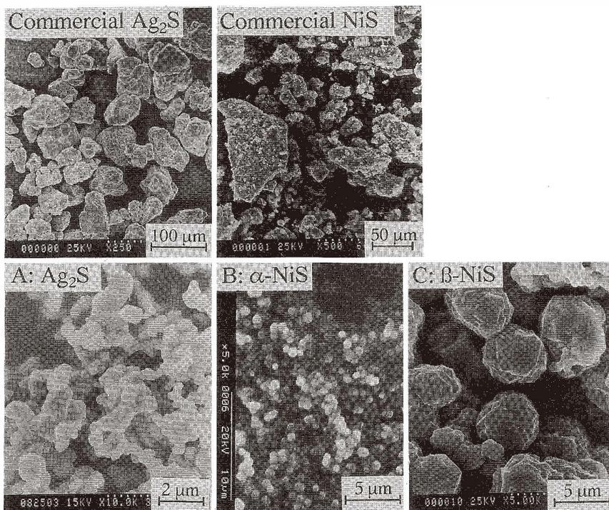
Fig. 2. SEM micrographs of commercial and synthesized metal sulfide particles. Reaction conditions are from Table 2.
