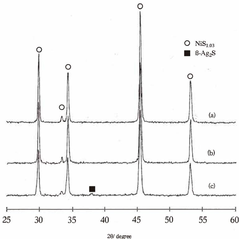
Fig. 4. X-ray diffraction patterns of raw NiS and  $\text{Ag}_2\text{S}$ -coated NiS particles. (a) raw NiS particles, (b)  $\text{Ag}_2\text{S}$ -coated NiS particles (coating time 0.5 h), and (c)  $\text{Ag}_2\text{S}$ -coated NiS particles (coating time 2.5 h).
