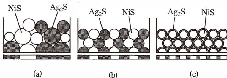
Fig. 1. Schematic models of electrode membranes. (a) large and rough  $\text{Ag}_2\text{S}$  and  $\text{NiS}$  particles, (b) monodispersed fine  $\text{Ag}_2\text{S}$  and  $\text{NiS}$  particles and (c) monodispersed fine  $\text{Ag}_2\text{S}$ -coated  $\text{NiS}$  particles.
