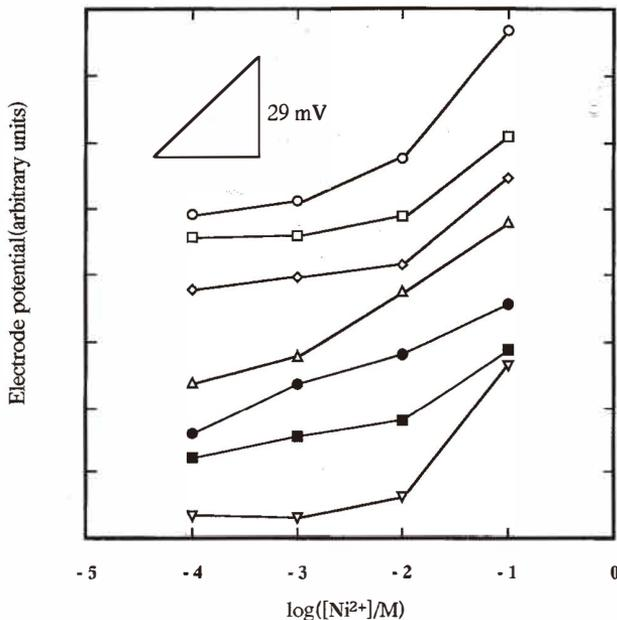
Fig. 6. Response of the electrodes fabricated using a mixture of synthesized  $\text{Ag}_2\text{S}$  and  $\beta$ -NiS particles at different weight ratios. Weight percent of  $\beta$ -NiS particles, ○: 25 wt%; □: 33 wt%; ◇: 50 wt%; △: 67 wt%; ●: 75 wt%; ■: 80 wt%; ▽: 91 wt%.
