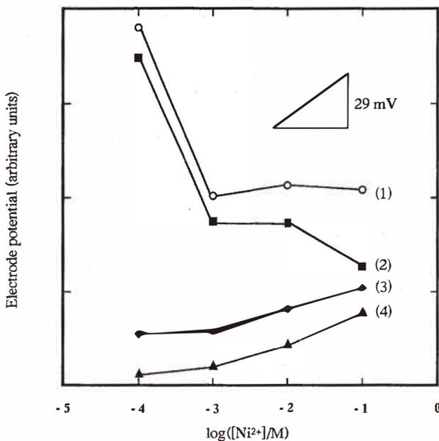
Fig. 5. Response of electrodes fabricated using a mixture of synthesized  $\text{Ag}_2\text{S}$  particles and synthesized NiS ( $\alpha$ -type) or commercial NiS ( $\gamma$ -type) particles. Type and weight percent of NiS particles: (1) commercial NiS(50 wt%); (2) synthesized  $\alpha$ -NiS(33 wt%); (3) synthesized  $\alpha$ -NiS(50 wt%); and (4) synthesized  $\alpha$ -NiS(67 wt%).
