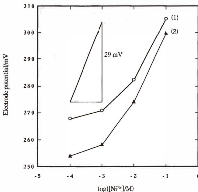
Fig. 7. Potential response of the electrodes fabricated using  $\text{Ag}_2\text{S}$ -coated NiS particles. Electrode (1): coating time 0.5 h, and electrode (2): coating time 2.5 h.
