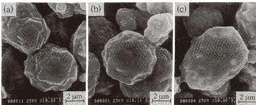
Fig. 3. SEM micrographs of Ag<sub>2</sub>S-coated NiS particles. (a) raw NiS particles, (b) Ag<sub>2</sub>S-coated NiS particles (coating time 0.5 h) and (c) Ag<sub>2</sub>S-coated NiS particles (coating time 2.5 h). Conditions of the coating reaction: amount of NiS particles: 0.0044 mol; amount of AgNO<sub>3</sub>: 0.0022 mol; reaction temperature: 0°C; solvent and volume: ethanol and 100 ml.
