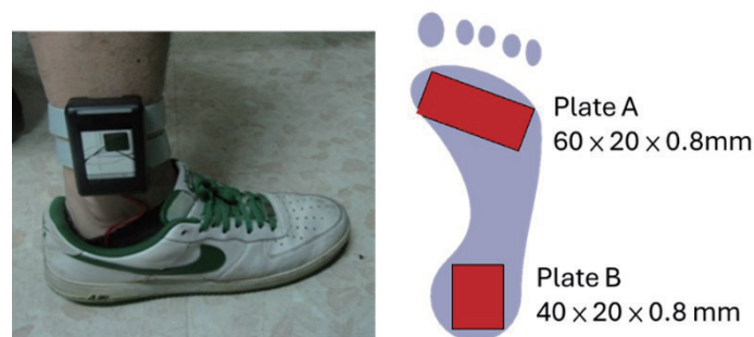
Fig. 2. (Color online) Placement of piezoelectric plates in the insole.
