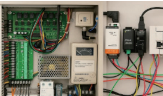
Fig. 11. (Color online) Architecture of PLC control box.
