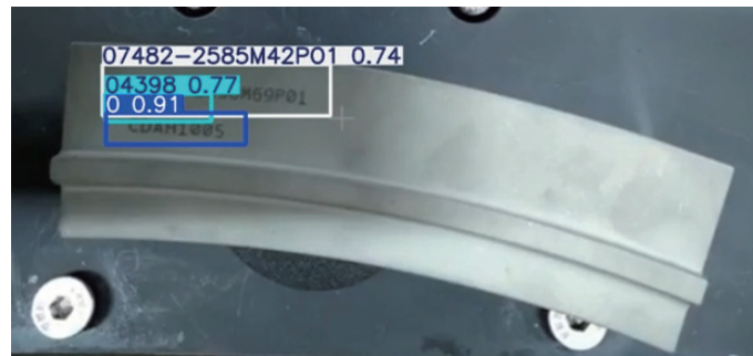
Fig. 8. (Color online) YOLOv8 detection results demonstrating accurate character localization.
