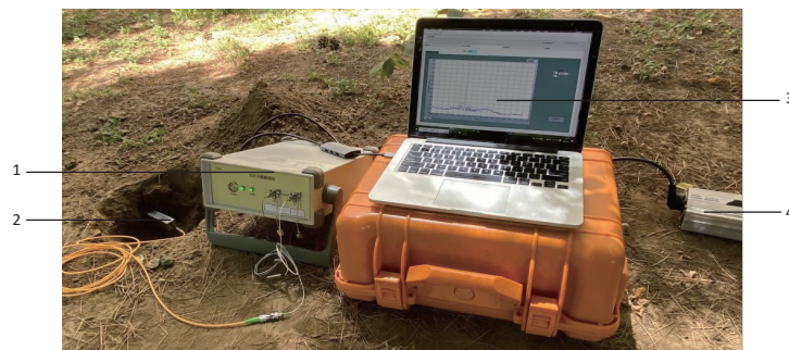
Fig. 13. (Color online) Practical application of the soil moisture measurement system. 1. Soil moisture sensor demodulation unit; 2. Soil moisture sensor unit; 3. Personal computer (PC); 4. Power supply.
