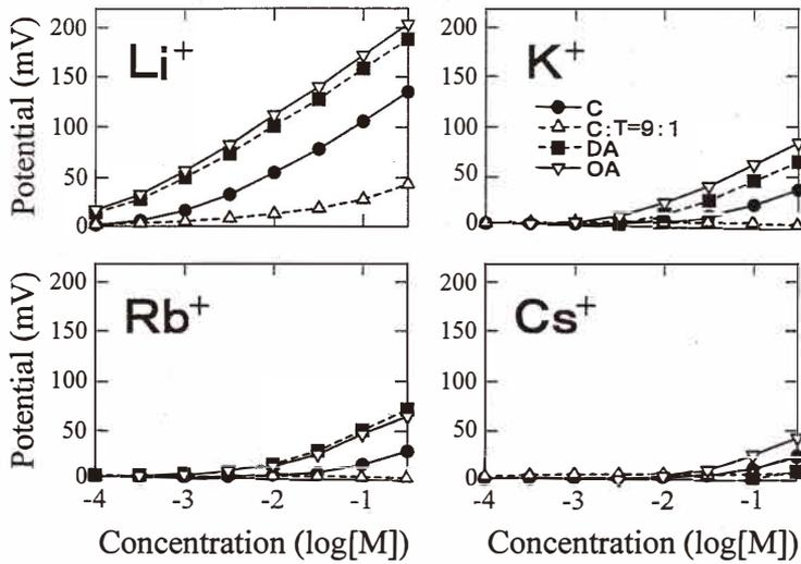
Fig. 4. Response curves of taste sensors to various monovalent cations.
