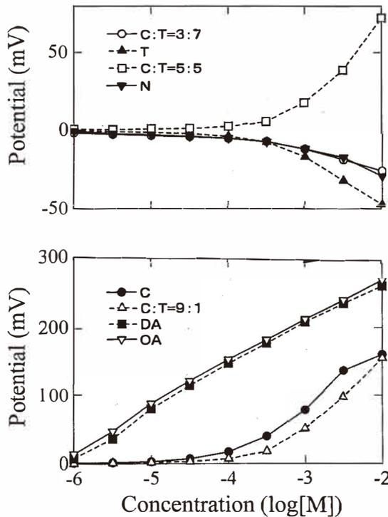
Fig. 2. Response curves of taste sensors to quinine hydrochloride.
