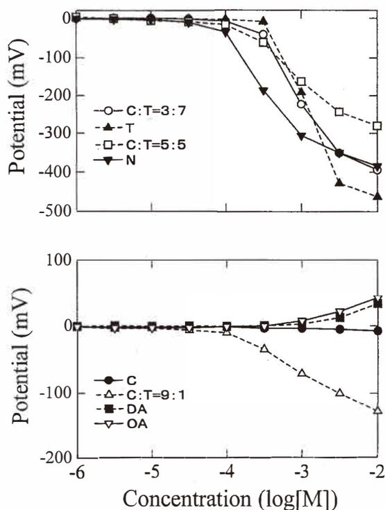
Fig. 3. Response curves of taste sensors to sodium picrate.
