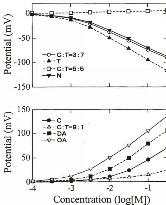
Fig. 1. Response curves of taste sensors to NaCl.
