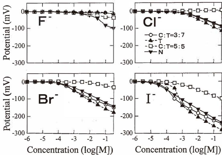
Fig. 5. Response curves of taste sensors to various monovalent anions.
