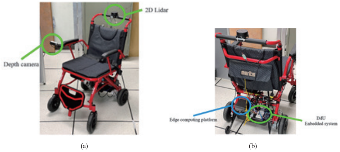
Fig. 7. (Color online) Exterior views of the intelligent wheelchair: (a) side and (b) rear views.
