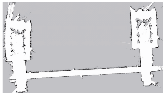
Fig. 8. SLAM result of the second floor of the Engineering Building.
