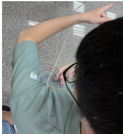
Fig. 17. (Color online) Angle \varphi_L measured using a protractor is 80^\circ .
