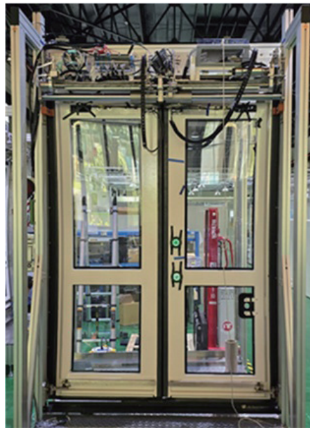
Fig. 10. (Color online) Physical view of the train door testing system.
