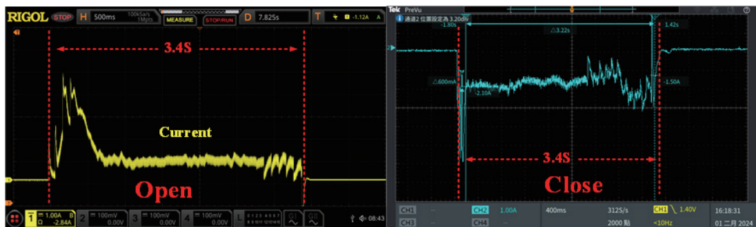
Fig. 11. (Color online) Real motor current waveforms during door opening and closing under variable-step speed control.
