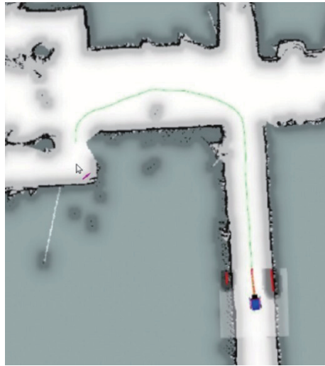
Fig. 13. (Color online) Mission map (green line is Dijkstra, red line is TEB).
