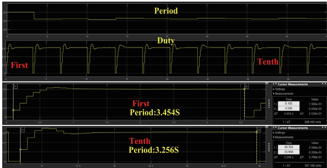
Fig. 8. (Color online) Convergence of door opening period through iterative variable-step speed control with triangular compensation.
