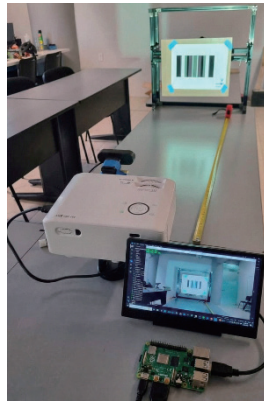
Fig. 4. (Color online) Photograph of the experimental setup used for validation tests, showing the fixed camera–projector configuration and the specimen mounted on a translational structure enabling controlled lateral displacement along the x -axis.
