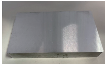
Fig. 4. (Color online) S45C medium-carbon steel workpiece used in grinding experiments.
