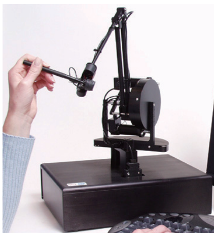
Fig. 3. (Color online) Example of a haptic device.
