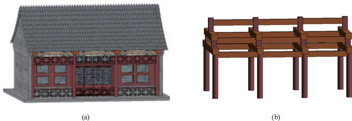
Fig. 8. (Color online) Five-purlin Small-style Building: a linear hall-type structure. (a) Overall view. (b) Detailed timber beam-frame structures.
