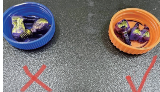
Fig. 13. (Color online) Visual representation of ceramic dental crowns specimens immersed in CV liquid solution for 15 min at room temperature. The cross mark ( \times ) indicates uncoated HA specimens and the check mark ( \checkmark ) indicates coated HA specimens.
