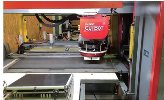
Fig. 3. (Color online) Turret-type automatic cutting machine.
