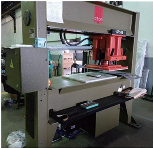
Fig. 2. (Color online) Energy-saving gantry cutting machine.
