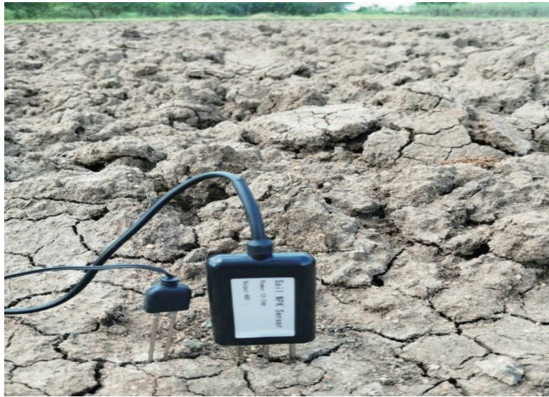
Fig. 6. (Color online) Soil condition testing under wet and dry environments.
