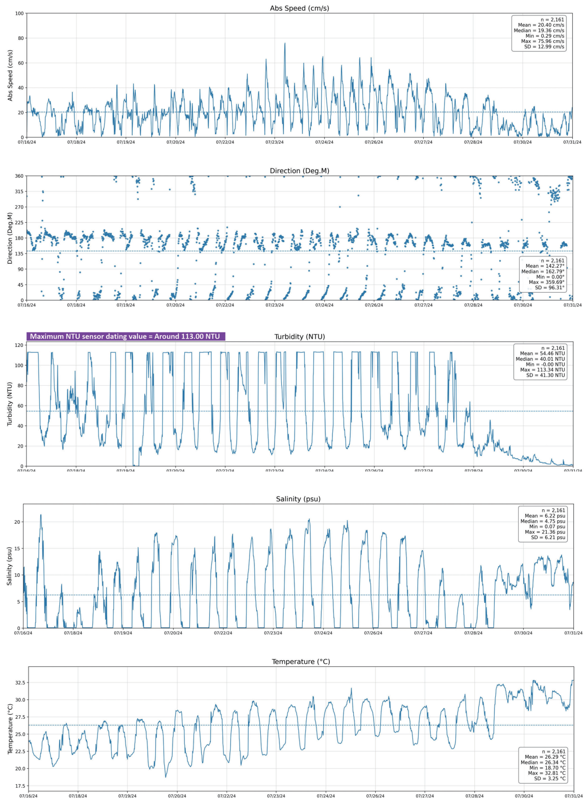
Fig. 7. (Color online) Station B-2 (July, flood season, fixed UV) time-series measurements of surface current velocity (speed), current direction, turbidity, salinity, and temperature; 16-day continuous physical dataset acquired.
