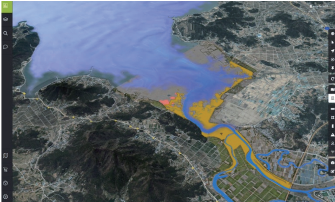
Fig. 11. (Color online) EGIS Inc. utilized a three-dimensional hydrodynamic SaaS-based numerical simulation model to conduct seawater circulation and salinity-dispersion simulations under both normal-flow and flood-season conditions in the Suncheon Bay estuary. (20)
