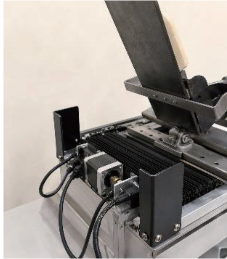
Fig. 16. (Color online) Front-mounted control cabinet support bracket of dual-axis CPM rehabilitation device.
