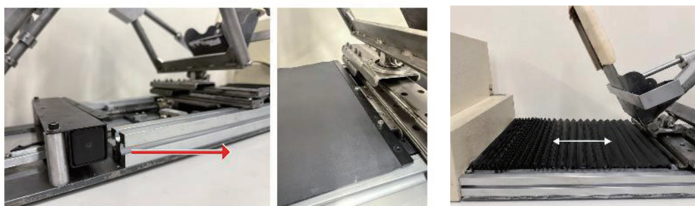
Fig. 15. (Color online) Installation of dustproof sleeve and protective cover on dual-axis CPM rehabilitation device to prevent dust intrusion and ensure operational safety during motion.
