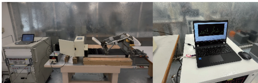
Fig. 17. (Color online) Functional testing setup of dual-axis CPM rehabilitation device, showing the control cabinet, HMI, and data monitoring through the connected laptop.
