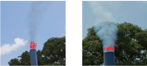
Fig. 9. (Color online) Eight small image patches are randomly sampled from the smoke region above the stack for opacity estimation.
