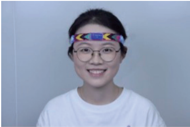
Fig. 2. (Color online) Photograph showing the BeneGear EEG headband positioned on a participant's forehead, with the copper-foil electrode pads in contact with the skin and the indicator light steadily on.
