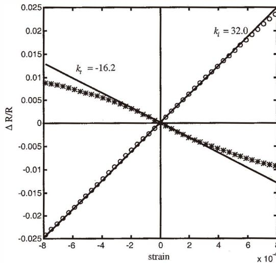
Fig. 7. Sensor response for undoped germanium.
