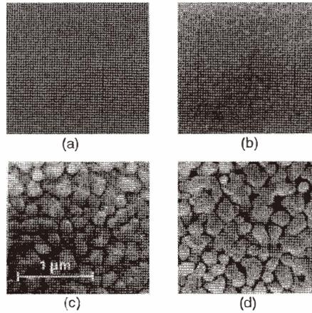
Fig. 1. SEM micrograph of the samples deposited at (a) room temperature, (b) 200°C, (c) 400°C and (d) 600°C.
