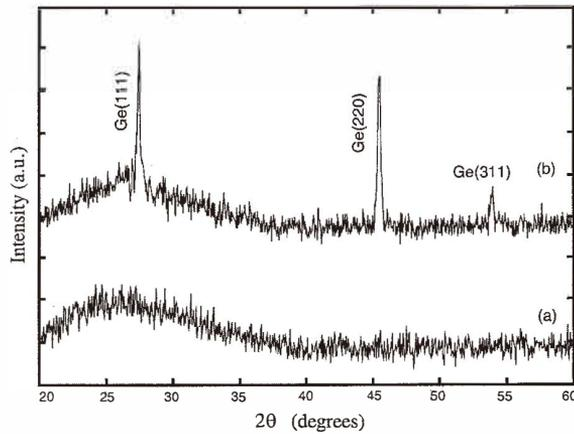
Fig. 2. XRD spectra of the samples grown at (a) room temperature (b) 400°C.
