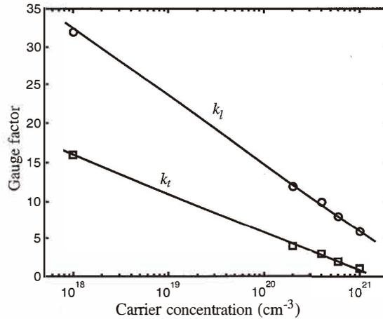
Fig. 8. Dependence of the longitudinal and transverse gauge factors on doping.
