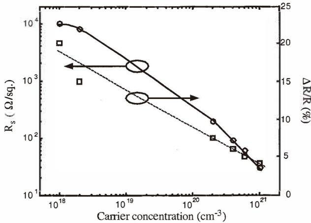
Fig. 5. Sheet resistance and its run-to-run variations as a function of the derived carrier concentration.
