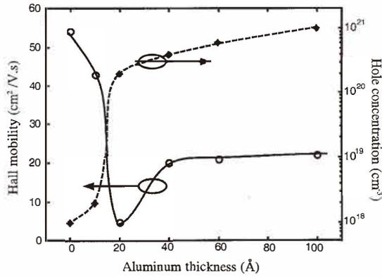
Fig. 4. Hole mobility and concentration determined from Hall measurements as a function of Al thickness.
