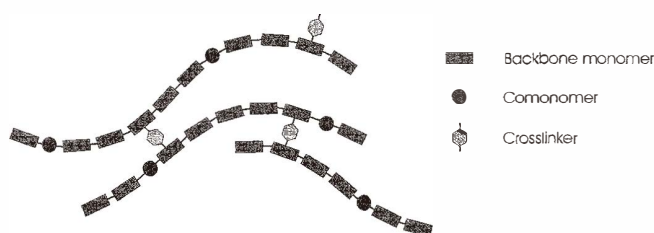
Fig. 1. Simplified view of the composition of a stimulus-sensitive hydrogel.
