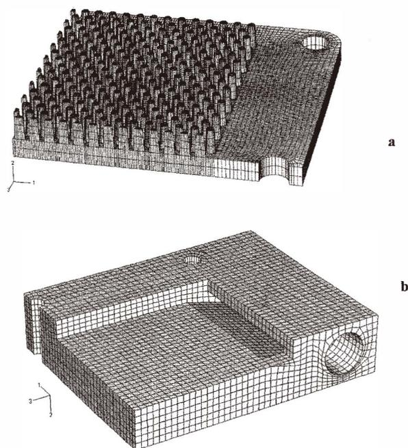
Fig. 3. 3D-finite element mesh (FEM) generated for the pin-fin heat sink (a) and for the channeling box (b).
