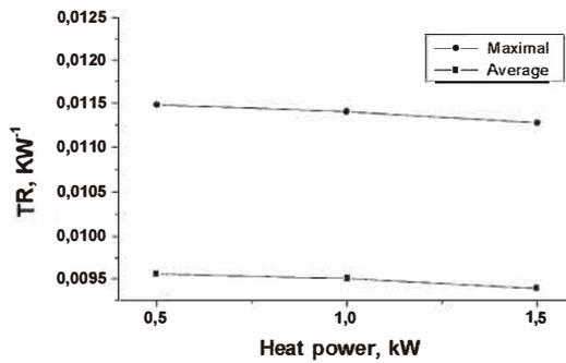
Fig. 11. Impact of heat power on final thermal resistance of the converter.
