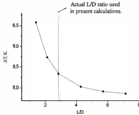
Fig. 15. Temperature difference between maximal temperature on the top surface of the simple model and inlet temperature of the cooling fluid  $T_{av}-T_0$  as a function of the ratio  $L/D$  (length of pin divided by its diameter).
