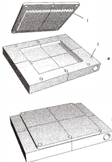
Fig. 1. Computer generated design of the cooling system for power semiconductor module: a) Disassembled heat converter: 1 - pin-fin sink, 2 - channeling box; b) Assembled heat converter.
