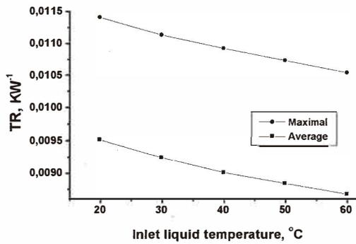
Fig. 10. Impact of inlet cooling fluid temperature on final thermal resistance of the converter.
