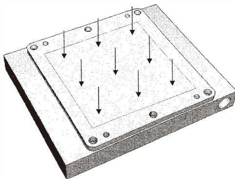
Fig. 5. Boundary condition: heat flux distribution at the top surface of the pin-fin sink.
