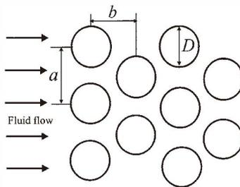
Fig. 2. Schematic of pin distribution at the pin-fin sink and specific geometrical parameters.
