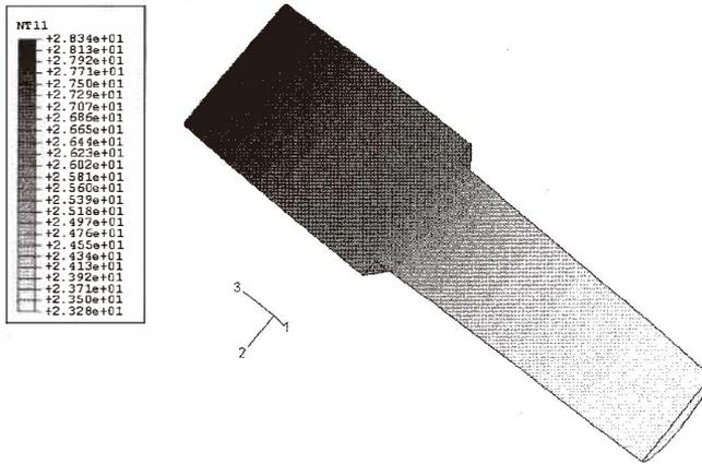
Fig. 13. Temperature distribution across the cross-section of the simple model.
