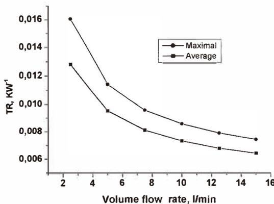
Fig. 8. Integral thermal resistance of the heat converter as a function of cooling fluid volume flow rate. Thermal resistances are calculated by means of eq. (5). Maximal for  $T^* = T^*_{max}$ , and average for  $T^* = T^*_{av}$ .
