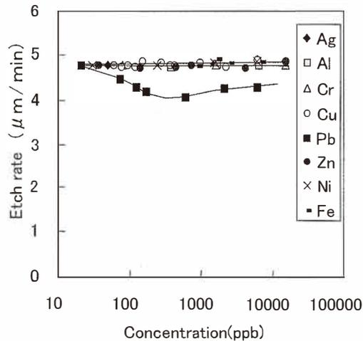
Fig. 2. Dependence of the etch rate of Si{100} plane on concentration of impurities (32wt% KOH, 110°C).
