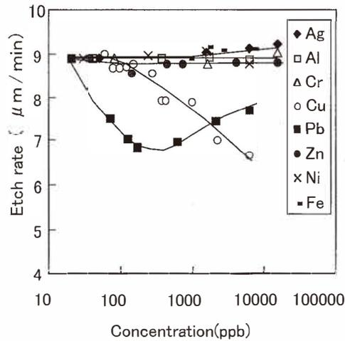
Fig. 1. Dependence of the etch rate of Si{110} plane on concentration of impurities (32wt% KOH, 110°C).
