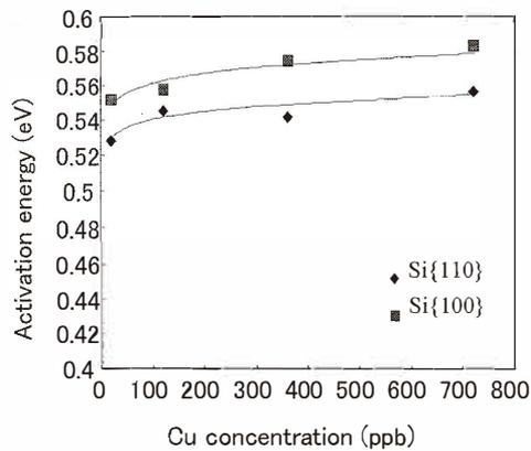
Fig. 5. Activation energies calculated for Si{110} and {100} in the solution containing ppb-level of Cu.
