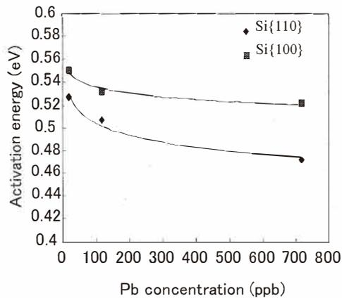
Fig. 6. Activation energies calculated for Si{110} and {100} in the solution containing ppb-level of Pb.
