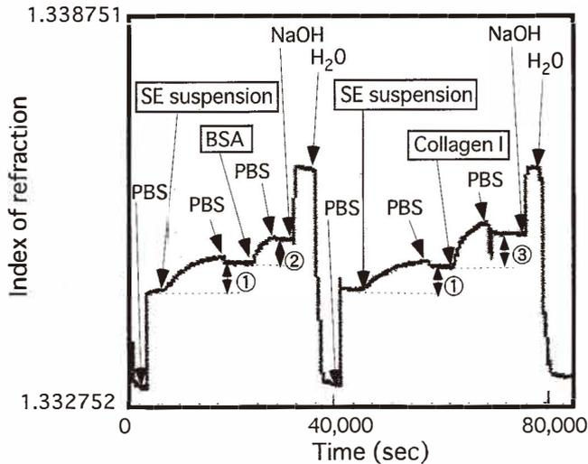
Fig. 2. Typical sensorgrams of *S. enteritidis* immobilization and the binding interactions of collagen I and BSA with the sensor surface immobilized with *S. enteritidis*. Solutions of collagen I and bovine serum albumin (BSA) were injected into the *S. enteritidis*-immobilized sensor surface in a volume of about 0.5 ml and the flow cell was washed and equilibrated with PBS. The RI was monitored.
