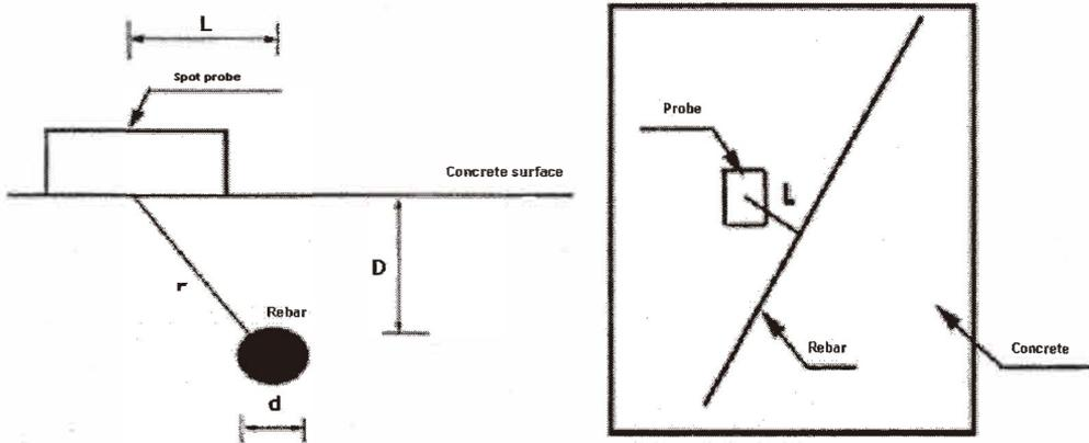
Fig. 3. Position of a covermeter probe on a concrete surface.
