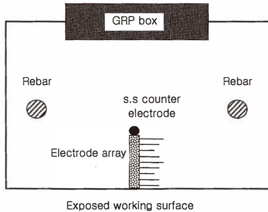
Fig. 7. Sectional view of covercrete array into the concrete.
