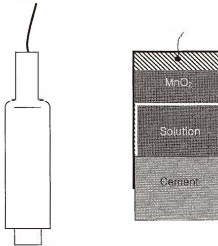
Fig. 8. Structure of  $\text{MnO}_2$  electrode.
