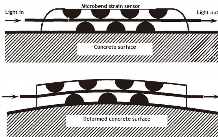
Fig. 5. Localized optical fiber sensor.
