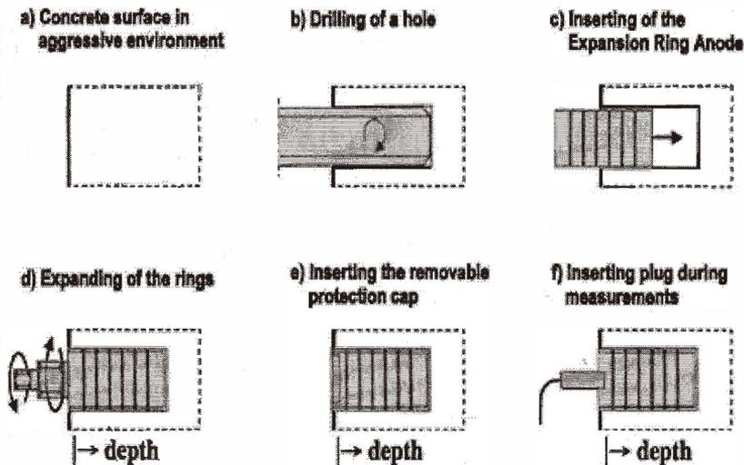
Fig. 2. Expansion-ring anode → installation procedure.
