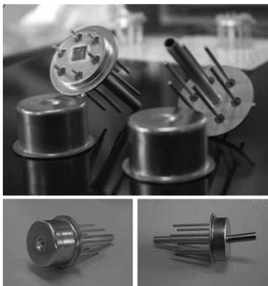
Fig. 6. Photographs of the packaged pressure sensors.
