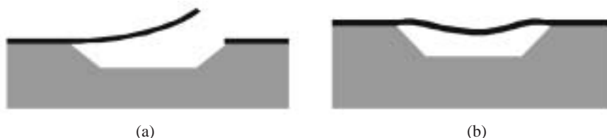
Fig. 2. Out-of-plane deformations: (a) microcantilever bending; and (b) microbridge buckling.
