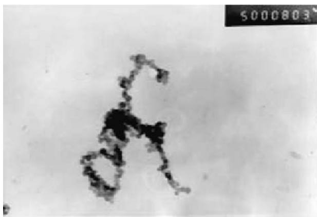
Fig. 2. TEM of \text{ZnFe}_2\text{O}_4 powder.
