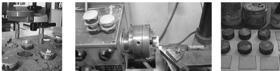
Fig. 16. DYNA, T. F. 16 kN, specimen preparation and rectification in pull-off tests.
