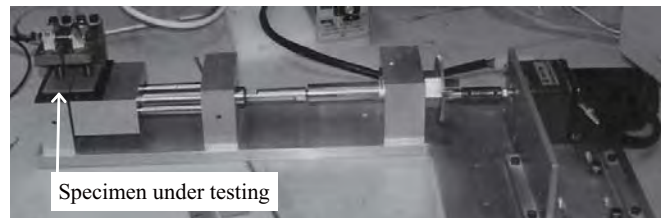
Fig. 7. Photograph of the mechanical crack simulator described by Leung et al. (9)
