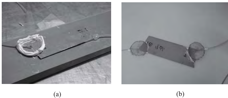
Fig. 18. Preparation of an embeddable plate sensor: (a) sealing of joint to protect the optical fibre and (b) plate sensor to be embedded.
