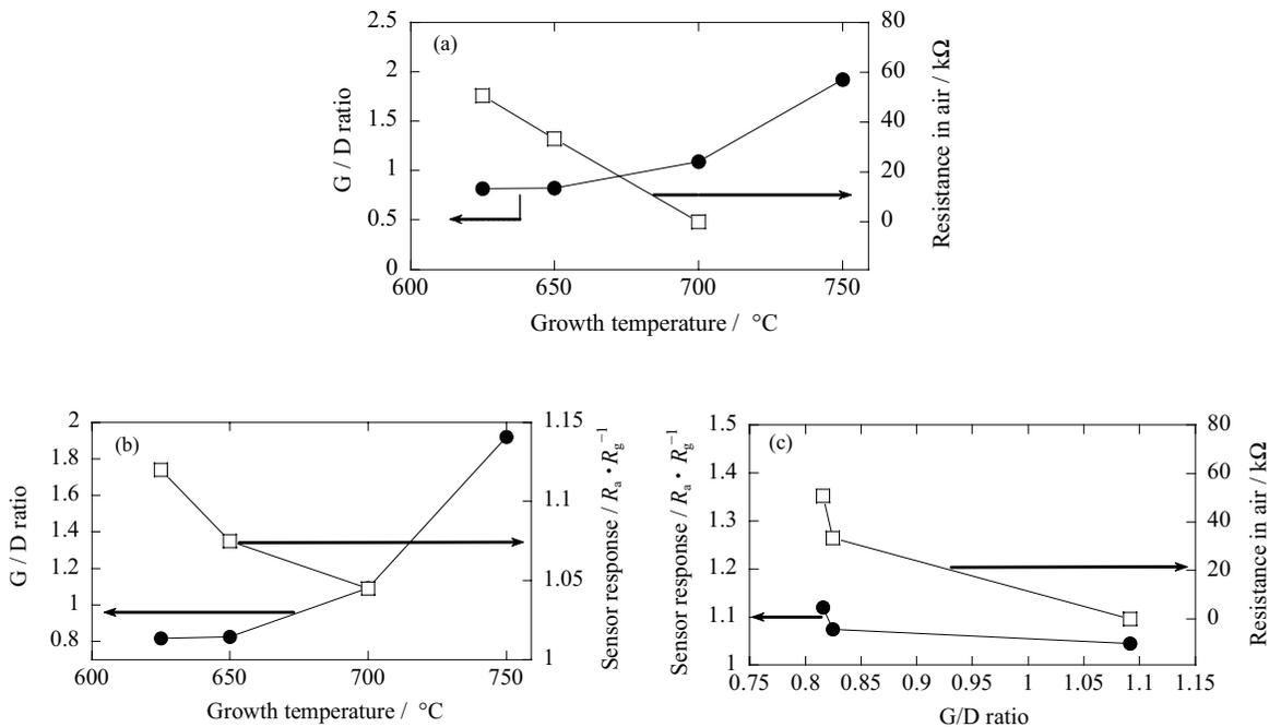
Fig. 5. Effects of growth temperature on (a) resistance in air and (b) sensor response of MWNT-based sensor to 5 ppm NO<sub>2</sub> at 100°C, and (c) dependence of resistance in air and sensor response on the G/D ratio of Raman shift of MWNTs.
