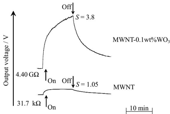
Fig. 11. Response transients of MWNT and MWNT-0.1 wt% WO<sub>3</sub> composite sensors to 5 ppm NO<sub>2</sub> at 200°C.
