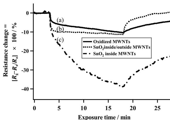
Fig. 15. Response transients of (a) oxidized MWNTs, (b)  $\text{SnO}_2$  inside/outside MWNTs and (c)  $\text{SnO}_2$  inside MWNTs to 1 ppm  $\text{NO}_2$  at  $150^\circ\text{C}$ .
