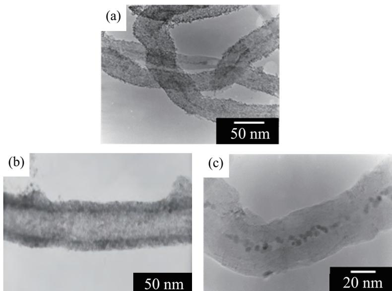
Fig. 13. TEM images of MWNT- $\text{SnO}_2$  composite fabricated by (a) calcination at 400°C for 3 h in air after washing with deionized water, (b) calcination at 400°C for 3 h in air and (c) calcination at 600°C for 3 h in argon and at 400°C for 3 h in air.
