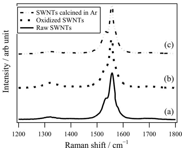
Fig. 14. Raman spectra of (a) raw SWNTs, (b) oxidized SWNTs and (c) SWNTs calcined at 600°C for 3 h in argon.
