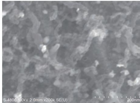
Fig. 2. SEM images of the 10- $\mu\text{m}$ -gap area of the MWNT-based sensor directly grown for 1 h at 700°C via ethanol CVD.
