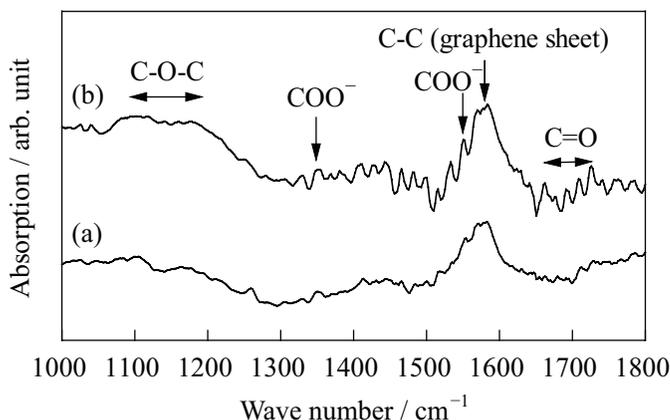
Fig. 8. Infrared absorption spectra of (a) MWNT and (b) oxidized MWNT.
