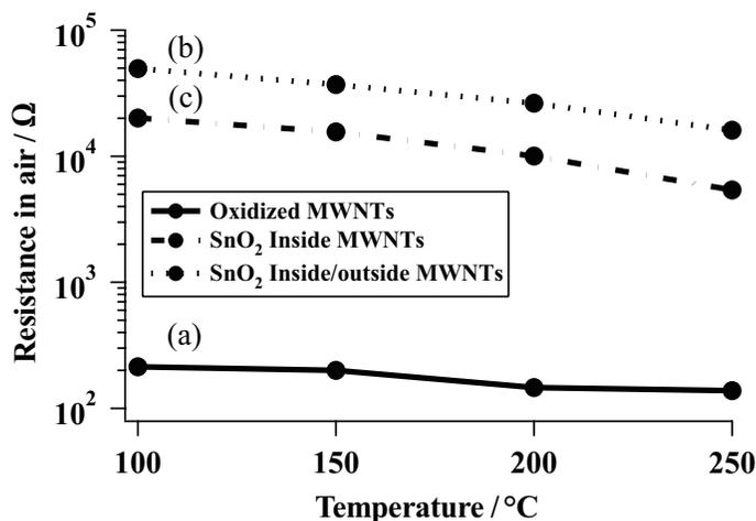
Fig. 16. Temperature dependences of resistance in air of (a) oxidized MWNTs, (b)  $\text{SnO}_2$  inside/outside MWNTs and (c)  $\text{SnO}_2$  inside MWNTs.
