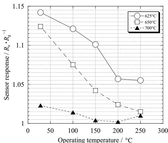
Fig. 6. Responses of MWNT-based sensors fabricated at growth temperatures of 625, 650, and 700°C to 5 ppm NO<sub>2</sub> as a function of operating temperature.
