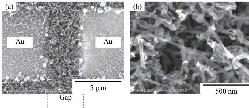
Fig. 9. SEM image of (a) MWNTs directly grown on Au microgap and magnified image of (b) entangled MWNTs between Au electrodes.
