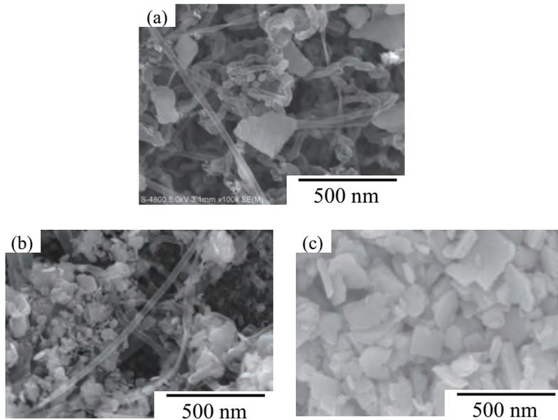
Fig. 10. SEM images of MWNT-WO<sub>3</sub> composite sensors obtained by argon calcination of MWNT-based sensor to which (a) 0.1, (b) 1 and (c) 7 wt% H<sub>2</sub>WO<sub>4</sub> suspensions were added.
