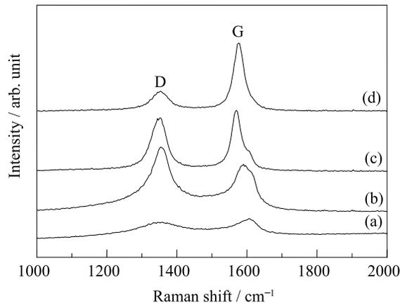
Fig. 4. Raman spectra of MWNT sensors grown for 1 h at (a) 625, (b) 650, (c) 700, and (d) 750°C via ethanol CVD.
