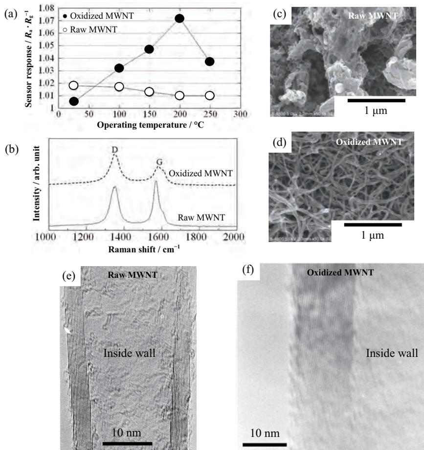
Fig. 7. Oxidation effects of MWNT on (a) sensor response to 5 ppm NO<sub>2</sub> as a function of operating temperature, (b) intensity of the G-band and the D-band in Raman spectra, (c, d) surface morphologies, and (e, f) roughness of sidewall.
