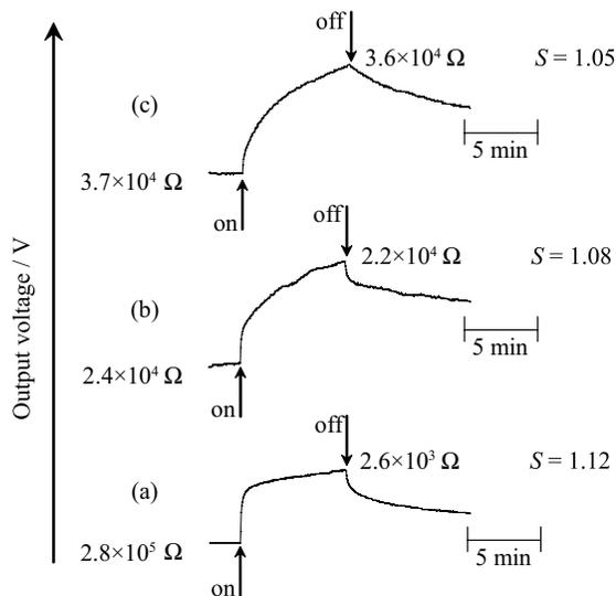
Fig. 3. Response transients of MWNT sensors to 5 ppm NO<sub>2</sub> in air at 100°C, which were grown for 1 h at (a) 625, (b) 650, and (c) 700°C via ethanol CVD.
