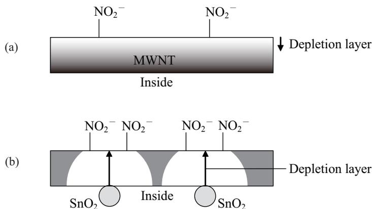
Fig. 17. Formation model of depletion layer in  $\text{NO}_2$  adsorption of (a) oxidized MWNT and (b)  $\text{SnO}_2$  deposited inside MWNT. A color gradation sequence from white to whitish gray denotes the depletion layer.
