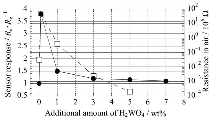
Fig. 12. Sensor response and resistance in air of MWNT-WO<sub>3</sub> composite sensors as a function of additional amount of H<sub>2</sub>WO<sub>4</sub>. (● Sensor response and □ Resistance in air)
