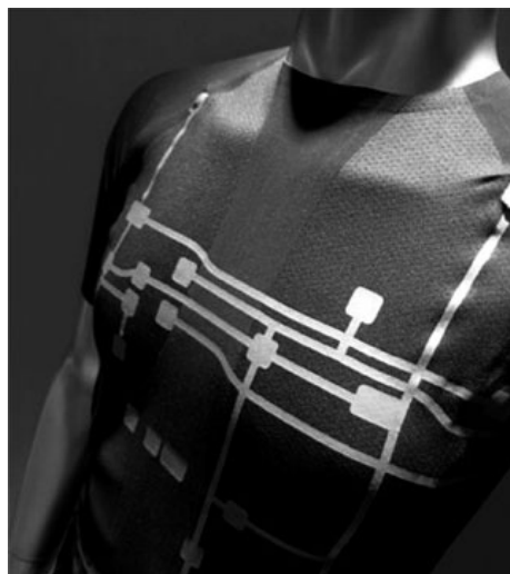
Fig. 1. Wearable ECG monitoring system with textile electrodes incorporated into a T-shirt, (1) recently commercialized by Biodevices S. A., in Portugal [ http://inventorspot.com/articles/wearable_heart_monitor_vital_jackets_fashionable_vital_monitorin_24622 ].
