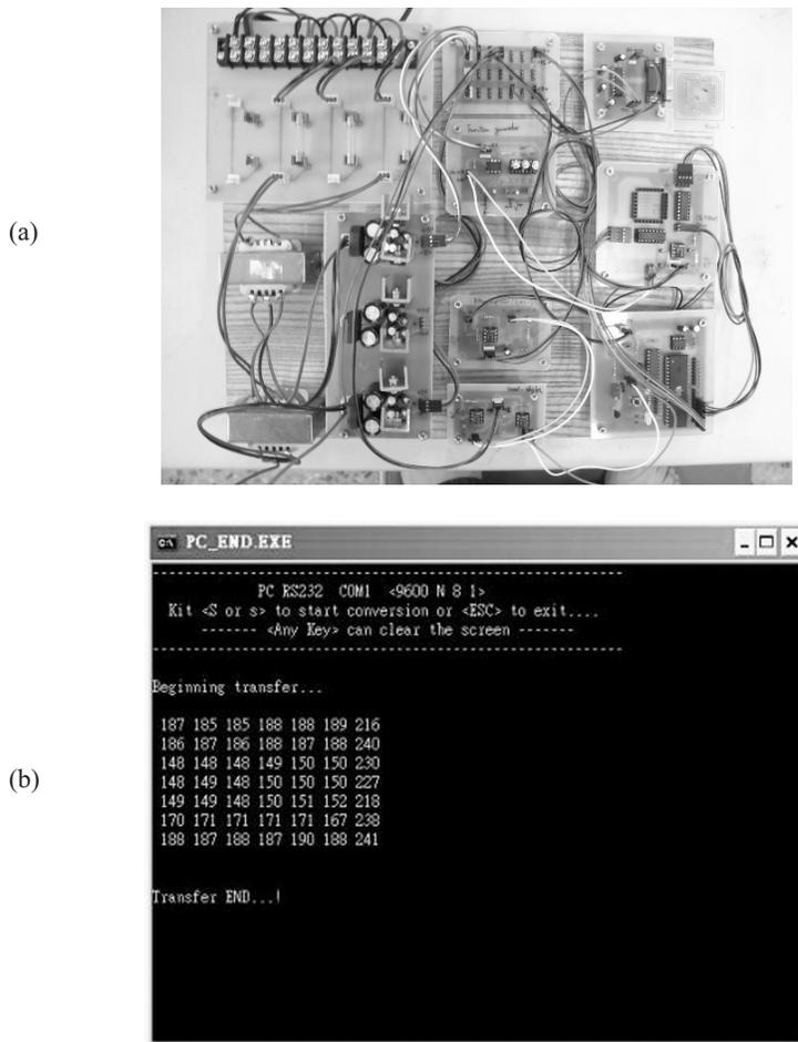
Fig. 6. Capacitance measurement using the detection system: (a) hardware of the measurement system and (b) capacitance signal displayed on the monitor.
