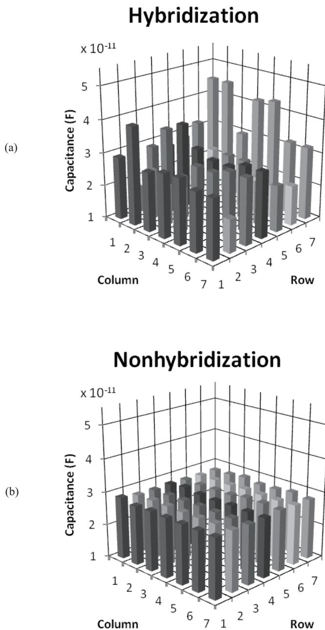
Fig. 7. Measured capacitances of the interdigitated electrode array for DNA (a) hybridization and (b) nonhybridization monitoring.
