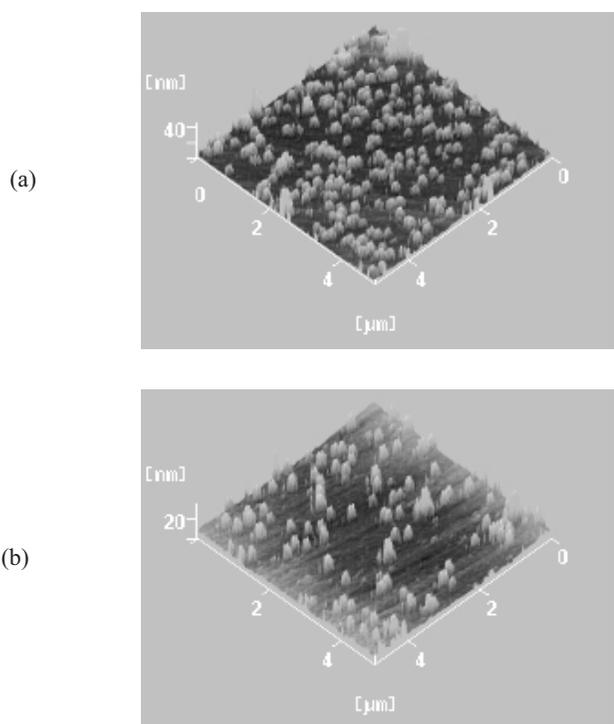
Fig. 5. AFM images of the interelectrode area: (a) hybridization surface and (b) nonhybridization surface.
