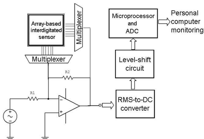
Fig. 3. Block diagram of the capacitance detection system.
