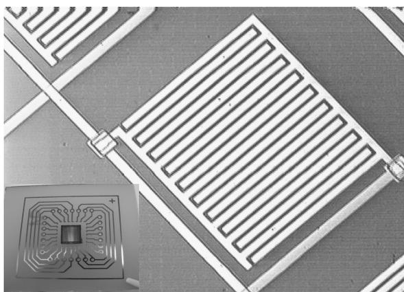
Fig. 4. Interdigitated sensing unit of the array chip. The inset shows a sensor array bonded on a PCB board.
