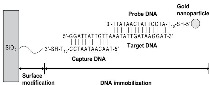
Fig. 2. Biomolecular structure of hybridized DNA on the silicon chip.
