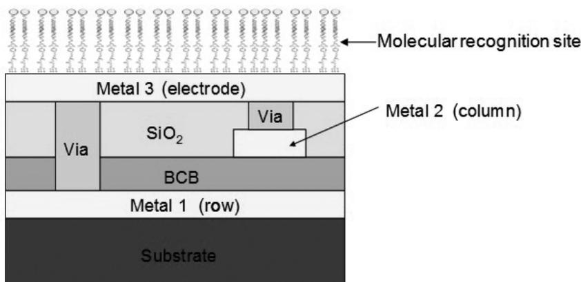
Fig. 1. Cross-sectional diagram of the interdigitated sensing chip.
