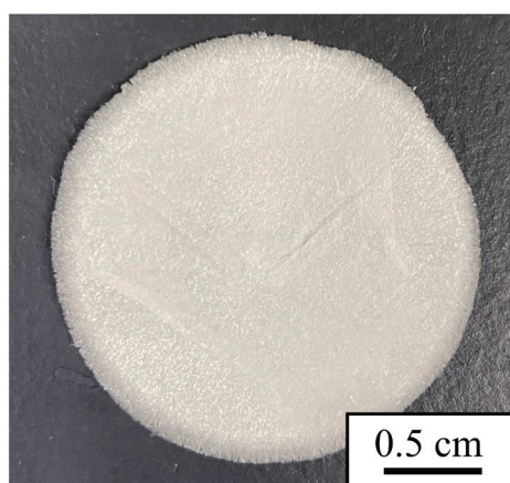
Fig. 2. (Color online) Sensor filter.
